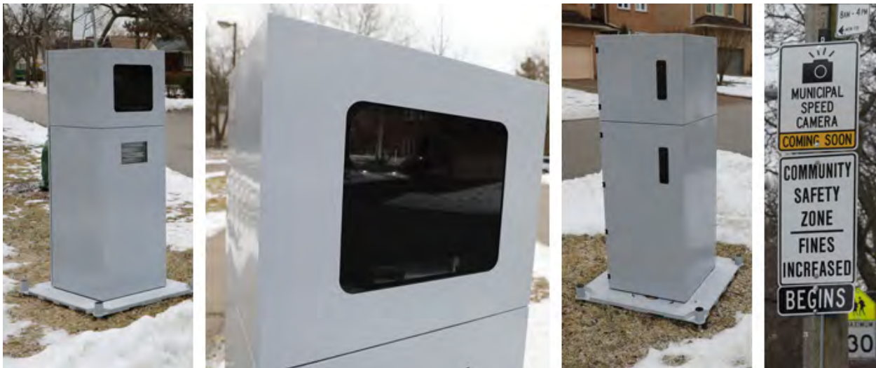
Figure 3-7: Automated Speed Enforcement Device and Corresponding Signage
