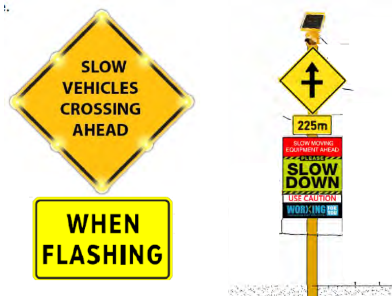
Figure 3-9: Slow Vehicles Crossing Ahead Signage and Warning System
