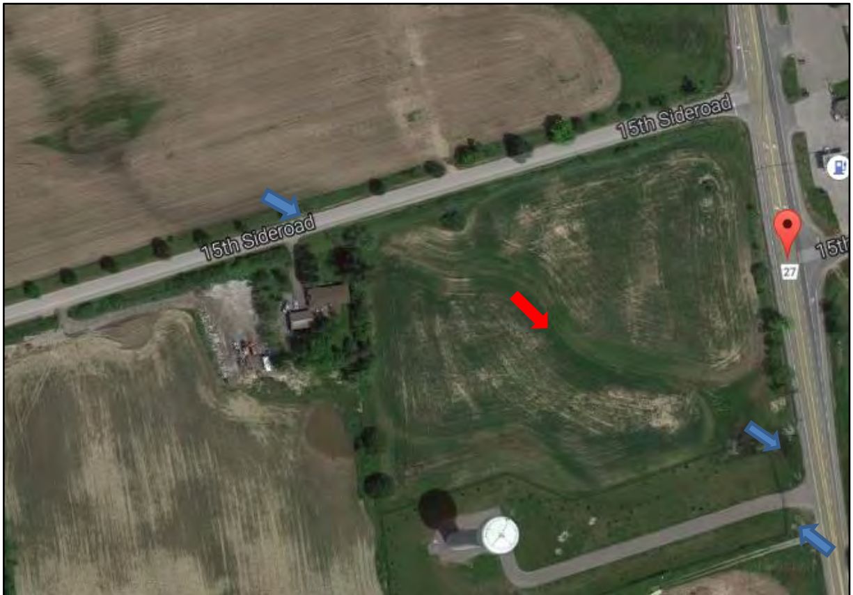
Map C. A Google Earth map of the site illustrating the drainage feature at 15 th Sideroad. The culverts are represented by the blue arrows and the red arrow represents drainage flow direction through the field.
