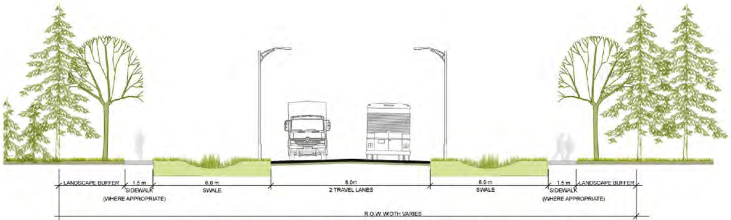
LOCAL ROAD THROUGH EMPLOYMENT AREA WITH SWALE
