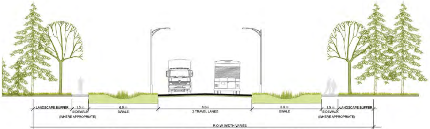
LOCAL ROAD THROUGH EMPLOYMENT AREA WITH SWALE
